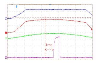
CH1: V<sub>LIVE</sub> (10V/DIV) CH2: Ampout (5V/DIV) CH3: I<sub>FAULT</sub> (10mA/DIV) CH4: Driver (1V/DIV)
