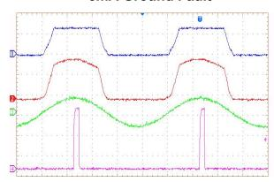
5mA Ground Fault (coil reverse)
