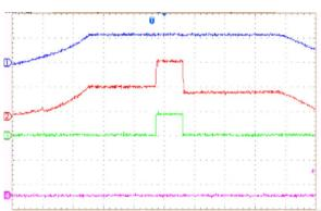
CH1: V<sub>LIVE</sub> (10V/DIV) CH2: Ampout (5V/DIV) CH3: I<sub>FAULT</sub> (20mA/DIV) CH4: Driver (1V/DIV)
